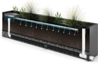
Water trickles through perforations into media.
