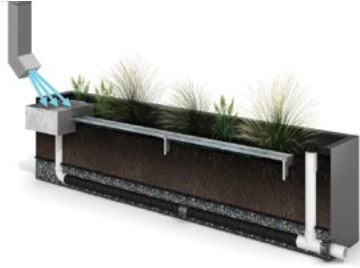
Water enters the Splash Box.
