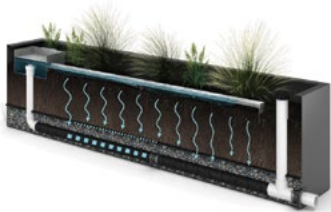
Water percolates through media and fabric.
