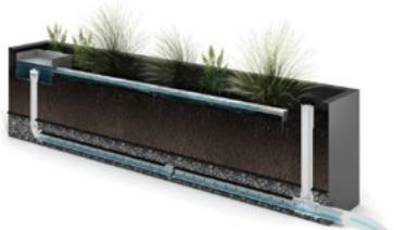
Water enters perforated drainpipe and exits.
