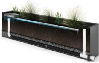
Water flows down the Level Spreader.
