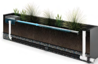
Water flows down the Level Spreader.
