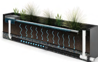
Water percolates through media and fabric.
